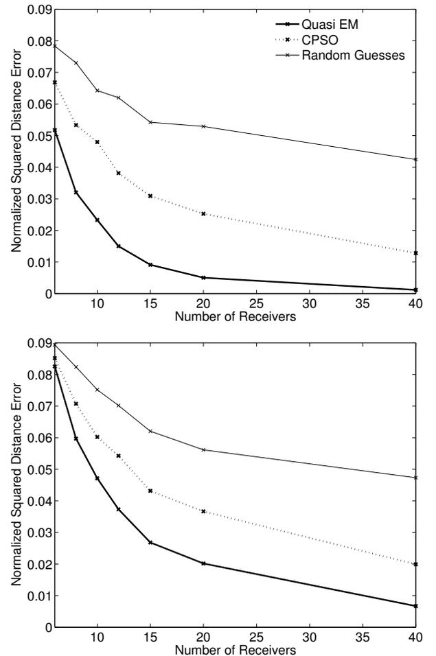
Fig. 3. Three transmitters: Median normalized average squared distance error for  $\sigma^2 = 4$  (top) and  $\sigma^2 = 16$  (bottom).
