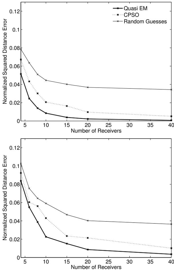
Fig. 2. Two transmitters: Median normalized average squared distance error for  $\sigma^2 = 4$  (top) and  $\sigma^2 = 16$  (bottom).
