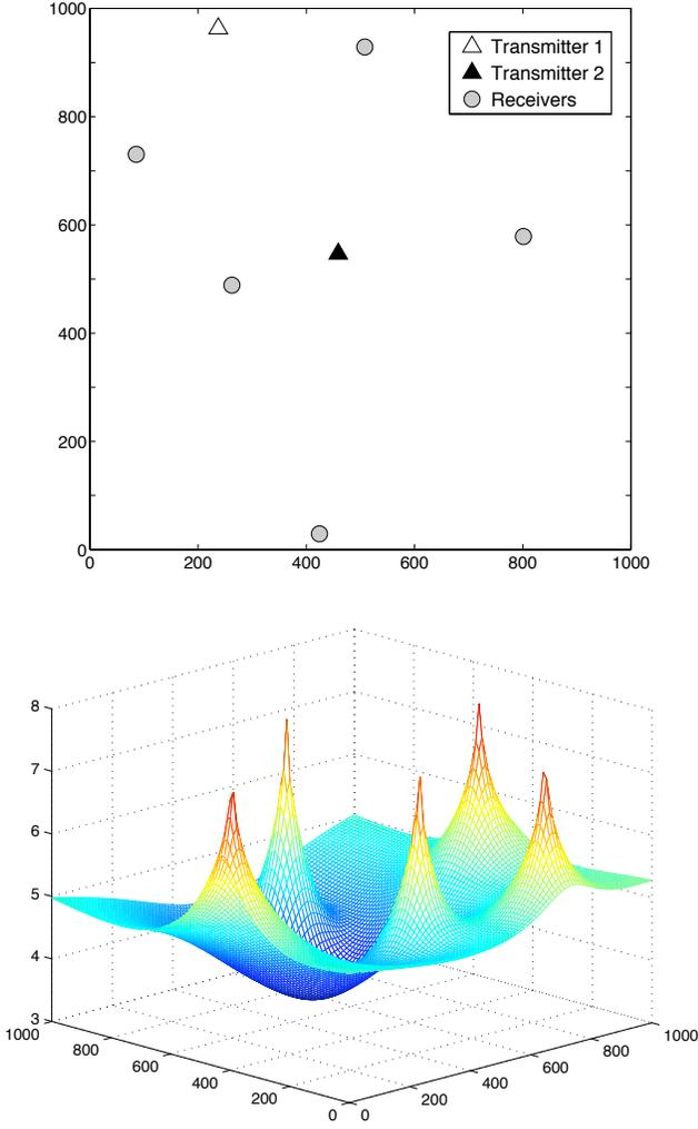
Fig. 1. **Top:** Example scenario for  $M = 2$  transmitters and  $N = 5$  receivers. **Bottom:** Associated scaled cost surface used to select the best estimate of transmitter 2's location when the location of transmitter 1 is estimated perfectly.
