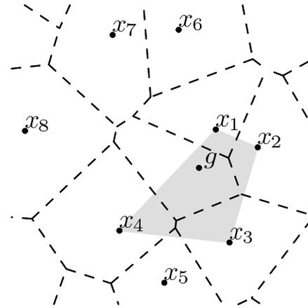
**Fig. 2.** Two-dimensional example of the enclosing k-NN neighbors of  $g$ ,  $\{x_i\}_{i=1,2,3,4}$ .
